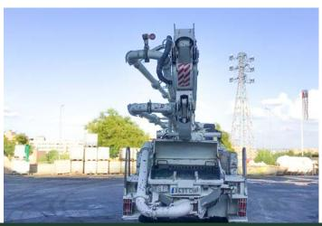
A four-armed, flexible and articulated boom provides great reach. The opening of the diagonal supports facilitates access to the concreting points. It is a compact machine with great manoeuvrability. Concrete lifting pump of 36 m. Mounted on a three-axle chassis. The Z-folding facilitates work in confined spaces with reduced heights. The pumping performance is twice as high as that of the 32 m. Pump.
